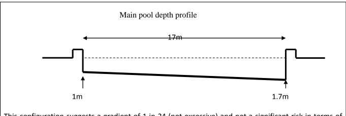
This configuration suggests a gradient of 1 in 24 (not excessive) and not a significant risk in terms of slipping.
